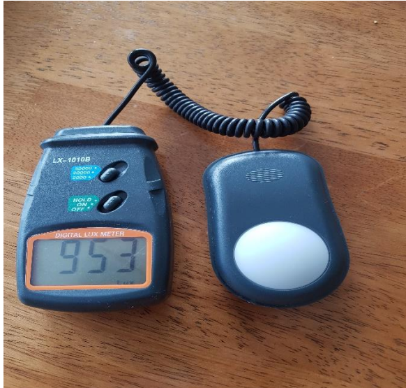
A portable light meter for measuring Lux levels
